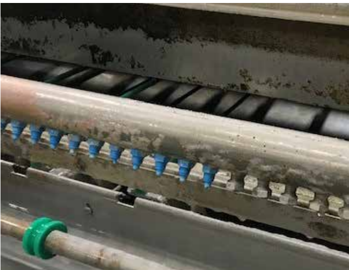
Spray nozzles are plugged with a heavy bio-slime. The biofilm is white in color and can be seen in the photo above the nozzles.
